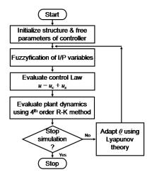
Fig. 2. Flowchart representation of LTBA of controller design.
