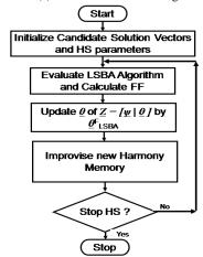
Fig. 4. Flowchart representation of hybrid concurrent algorithm of controller design.
