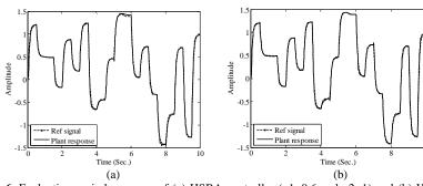
**Fig. 6.** Evaluation period response of (a) HSBA controller (n1=0.6 and n2=1) and (b) HCBA controller (n1=1.4 and n2=0.6).
